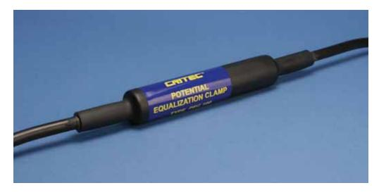
The PEC is an equipotential bonding device that can be used to minimise damage in applications where separated ground systems are required. The PEC100 model is ATEX approved making the device suitable for use in explosion hazard areas such as the protection of pipeline insulated joints. The PEC150 model is a higher surge rated product for more exposed locations subject to partial direct lightning strike.
